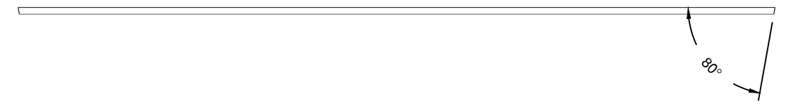
2 FRONT VIEW: PLYWOOD 1104 TWO SIDES AND FRONT ARE BEVELED 10 deg. 3/4"=1'-0" 3/4" CDX PLY
